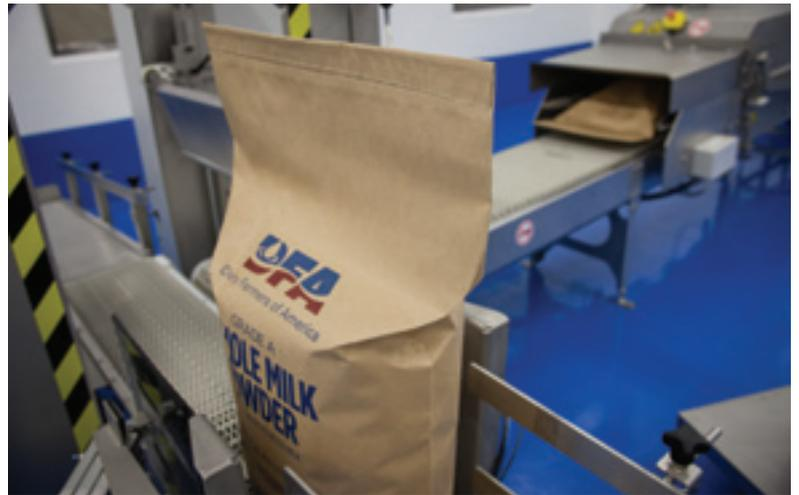
■ Employees at DFA's new milk powder plant in Fallon, Nev., can fill six 25-kilogram, oxygen-free bags of powder every minute. These are trucked to Oakland, Calif., and loaded on container ships bound for China and other countries.
